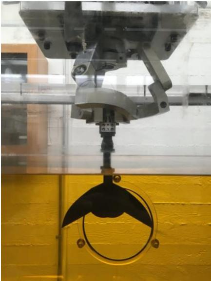
To test the fin, it is first attached to a force sensor via an adapter CADed on the top of the shell. The three robotic arms outside of the tank are the driving force behind the fin's movements. They can provide a large range of motion, so many types and variations of fin trajectories can be tested. During the movements, the forces on the fin are measured and recorded.
